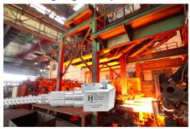
Our Triaxial series has expanded with the HS-173HT accelerometer being the latest addition to the range. This Triaxial features a 5 Core PTFE Cable with Stainless Steel Protective Conduit, and can withstand up to 150°C, with an acceleration and temperature output.
