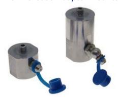
To improve the process when mounting the sensor with stud or magnet to the machine, we have introduced grease adaptor mounts. The HS-AS241 grease adaptor mount with 1/4"-28 UNF female accelerometer mounting thread, ensures accuracy and top cleanliness, producing an airtight seal.
