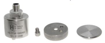
To enhance the fitting of a triaxial we have designed the HS-AS221 triaxial accelerometer adapter with Ø42mm knurled quick release, 1/4"-28UNF mounting.
